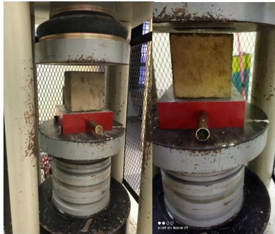
Figure 5: Compressive strength test
