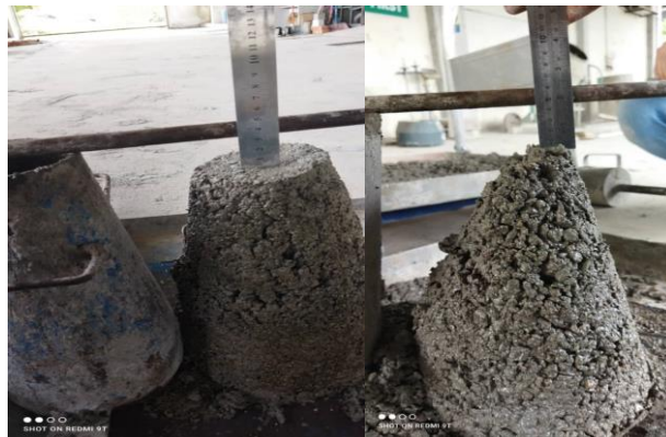
Figure 3: The slump test of different percentages of alum sludge
