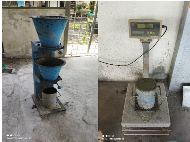
Figure 4: Compaction factor test
